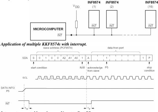
Interrupt generated by a change of input to Port P5.
